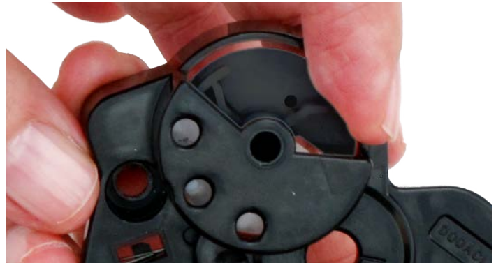
Figure 15-4: Turning the reset gear into place (1 of 2)
