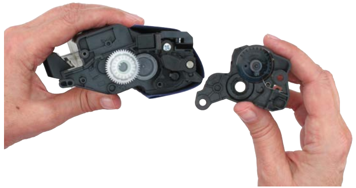
Figure 6-3: Remove the cartridge end cap
