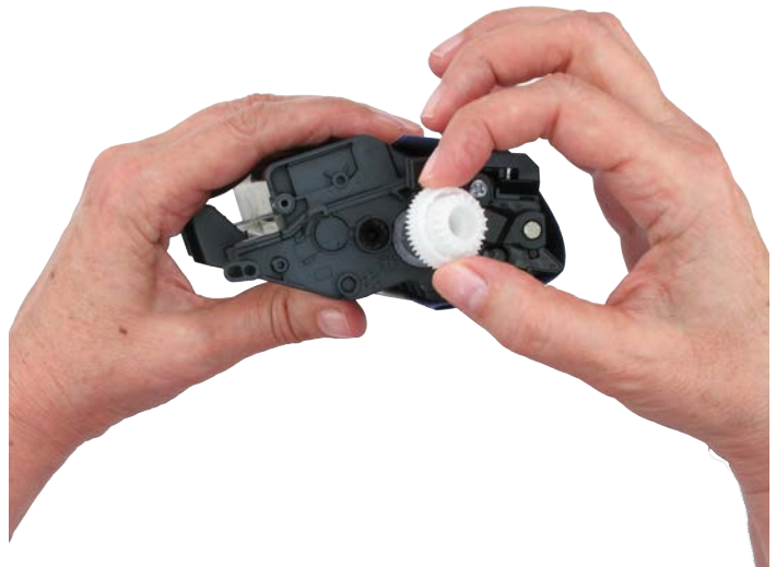
Figure 6-4: Remove the drive gear from the cartridge
