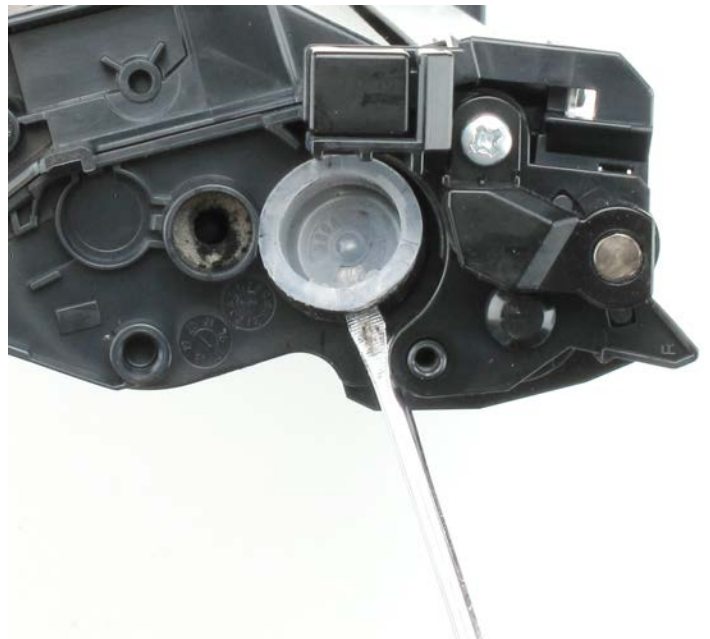
Figure 7: Removing the cartridge plug
