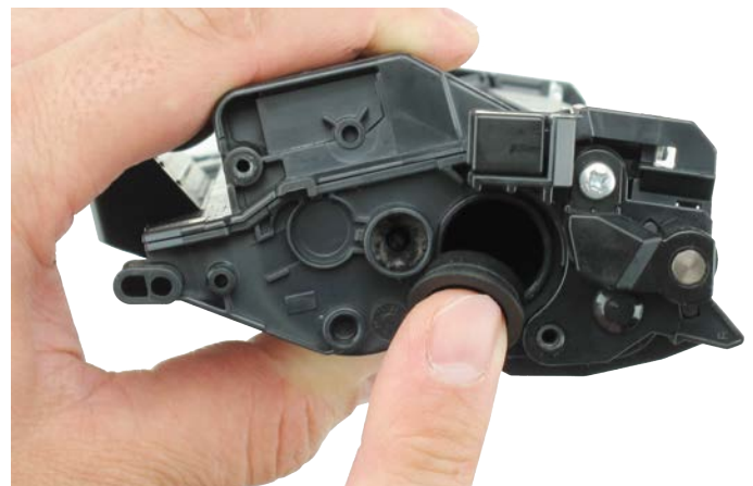
Figure 12: Applying the plug to the toner cartridge
