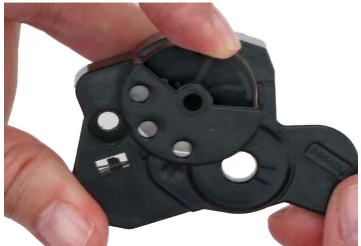
Figure 15-7: Rotating the gear the rest of the way (final position)
