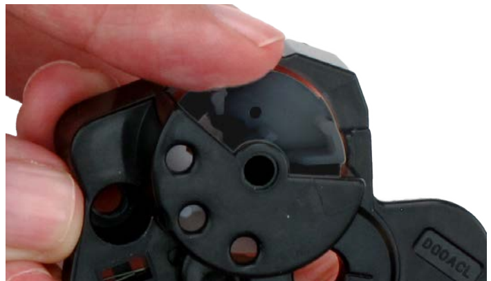
Figure 15-5: Turning the reset gear counterclockwise
