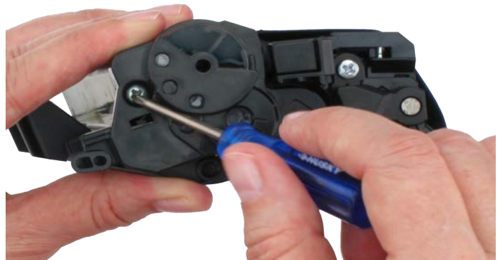
Figure 16-2: Reapplying the end cap screw (2 of 2)
