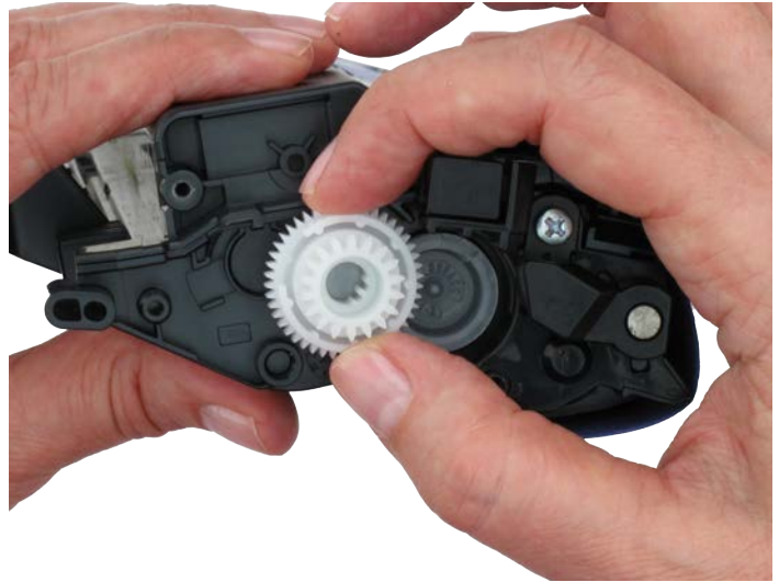
Figure 13: Placing the drive gear onto the cartridge
