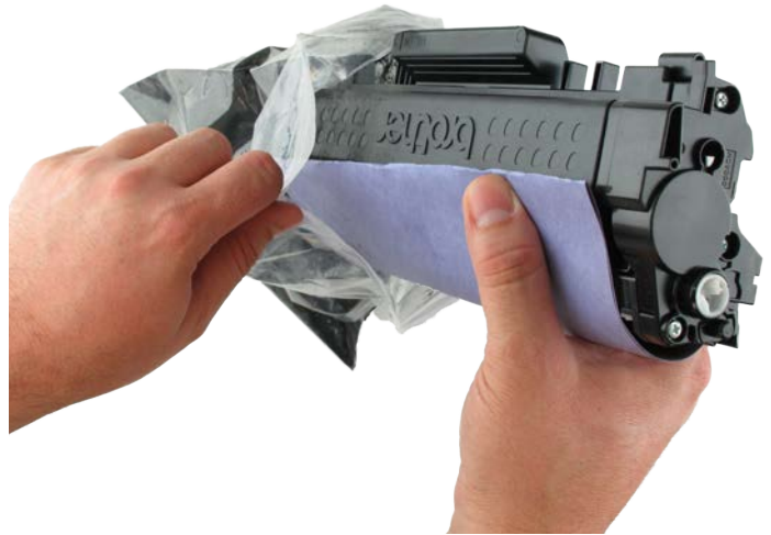
Figure 8: Removing the remaining toner from the cartridge
