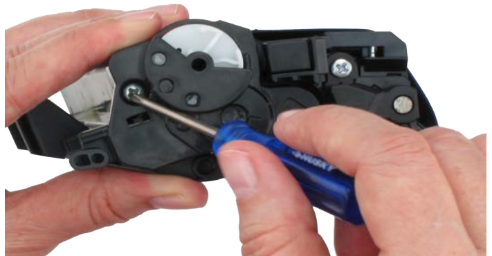
Figure 16-2: Reapplying the end cap screw (2 of 2)
