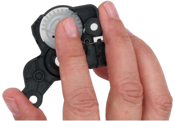
Figure 15-2: Securing the reset gear to the end cap
