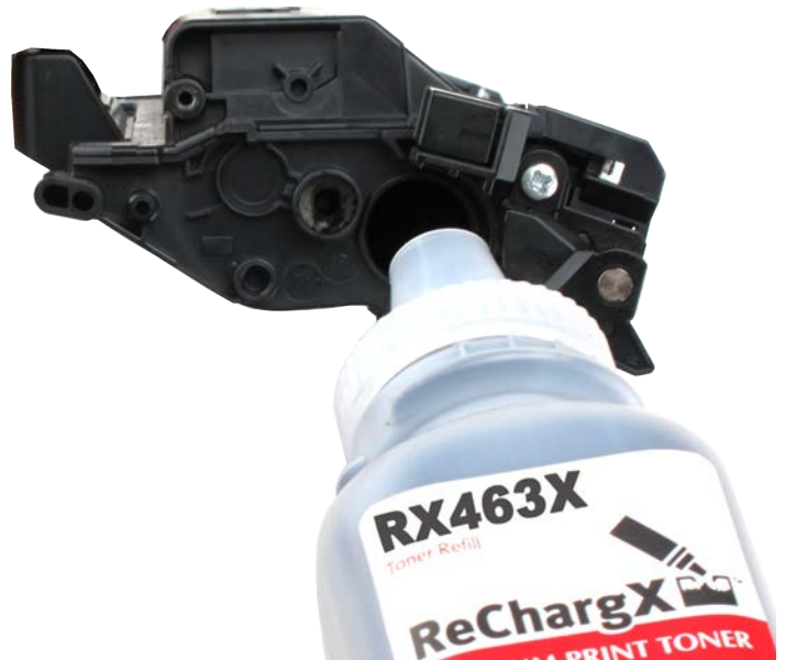
Figure 9: Refilling the toner cartridge
