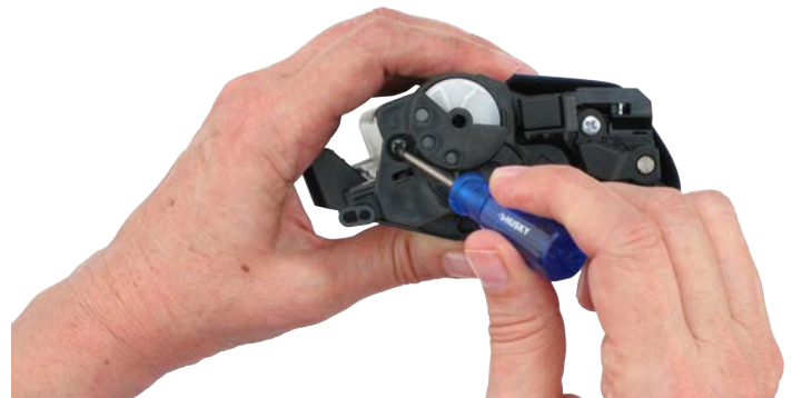
Figure 6-2: Removing the end cap screws (2 of 2)
