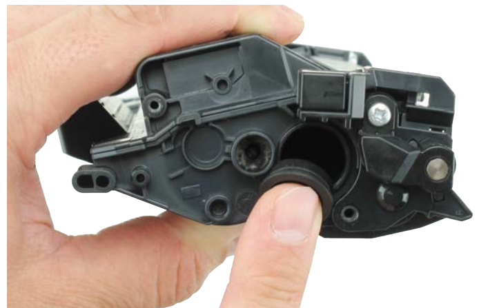
Figure 12: Applying the plug to the toner cartridge
