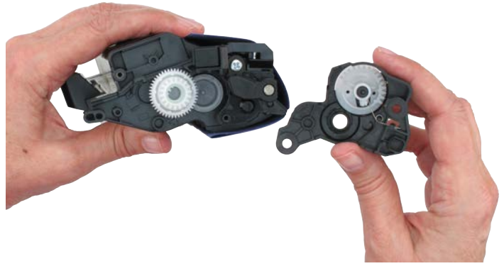
Figure 6-3: Remove the cartridge end cap
