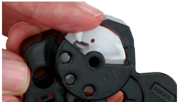
Figure 15-5: Turning the reset gear counterclockwise
