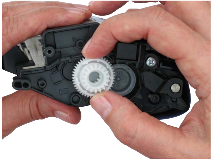
Figure 13: Placing the drive gear onto the cartridge
