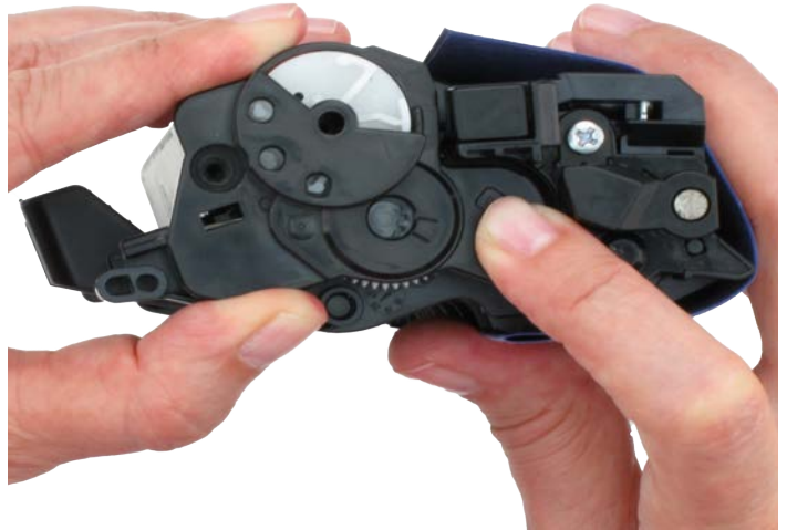
Figure 15-9: Securing the end cap to the toner cartridge
