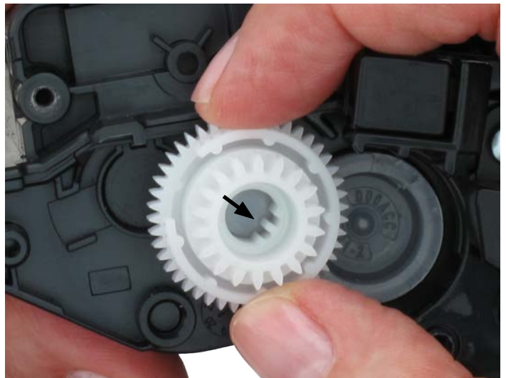
Figure 14: The drive gear in its reset position
