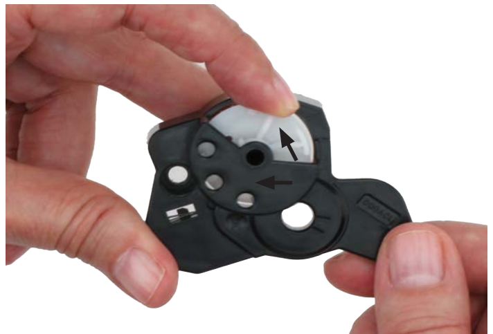
Figure 15-4: Rotate the gear the rest of the way (final position)
