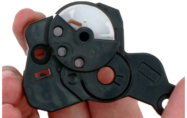
Figure 15-3: Hold the back of the reset gear, flip over
