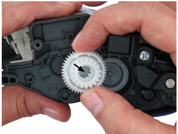
Figure 14: The drive gear in its reset position
